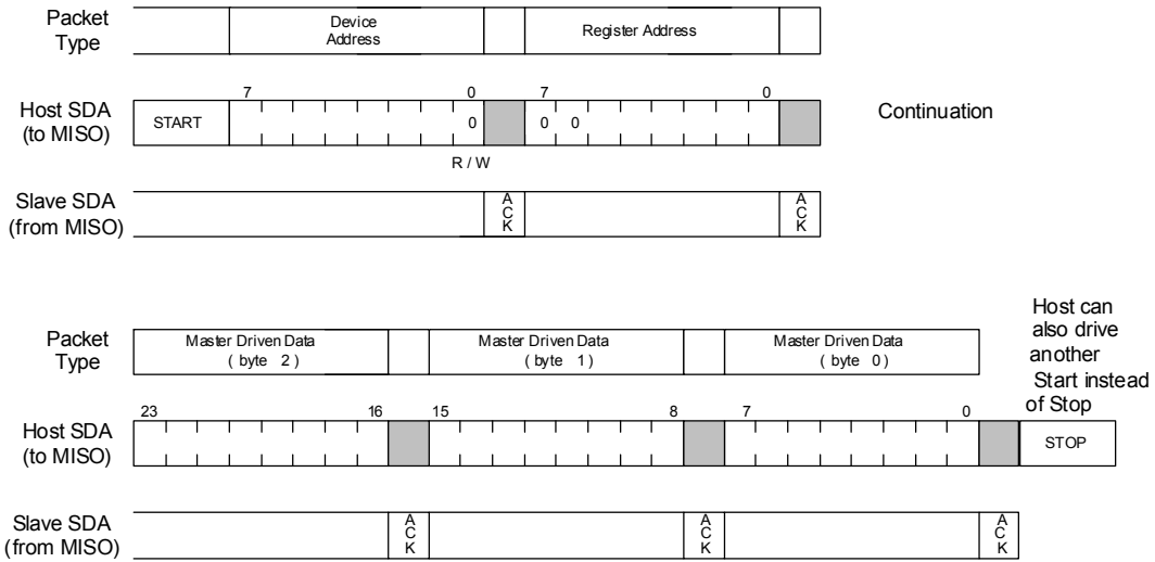
Figure 36. I 2 C 3-byte Write Example
